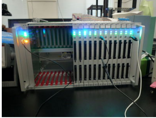
Figure 2.22: Photograph of a crate with a test pulse board and some power supply boards.
