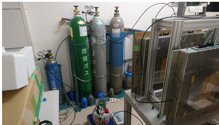
Figure 2.12: Photograph of the system flowing mixed gas to the multi-wire proportional chambers.
