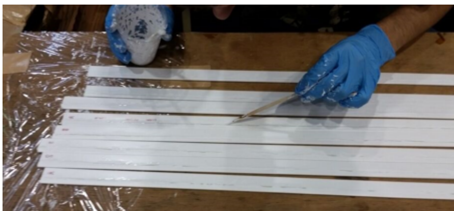
Figure 7.2.3: Fiber painting work
