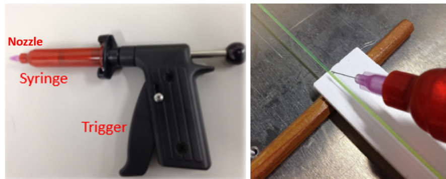
Figure 8.2.8: DispensGun ® : The light figure shows the nozzle for discharging the optical cement.
