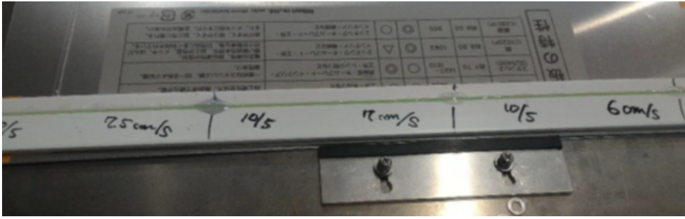
Figure 8.3.5: Test gluing work under a variety of velocity conditions
