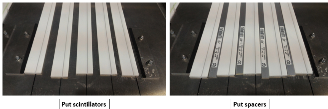
Figure 8.4.2: Setting spacers between scintillators
