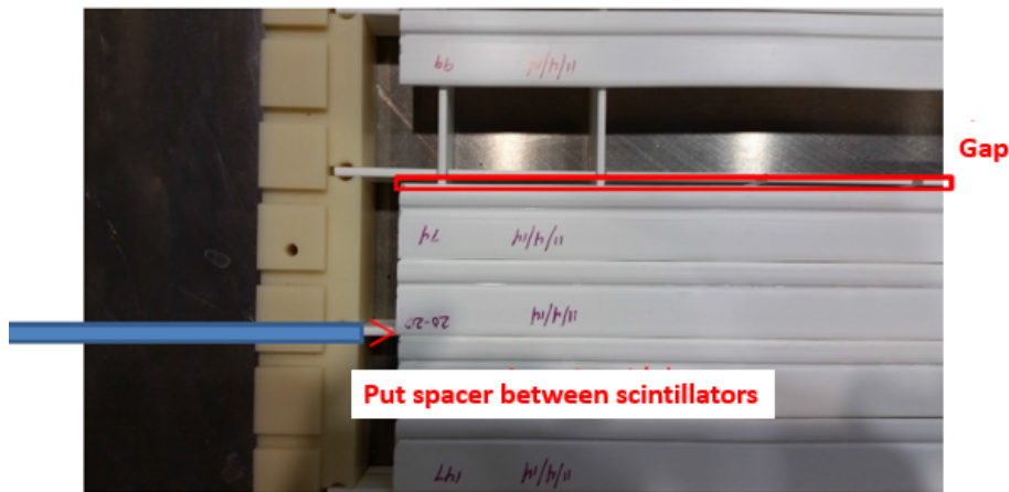
Figure 9.1.2: Put spacers between each scintillator
