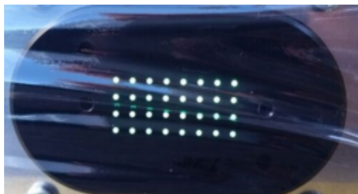
Figure 6.3.17: Polished fiber bundle
