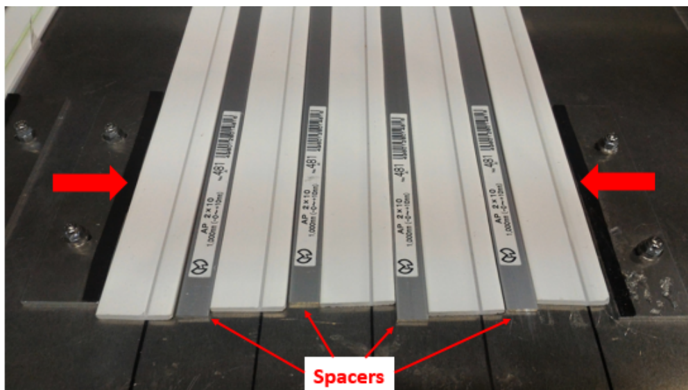
Figure 8.3.3: Jigs for fixing scintillator linearly
