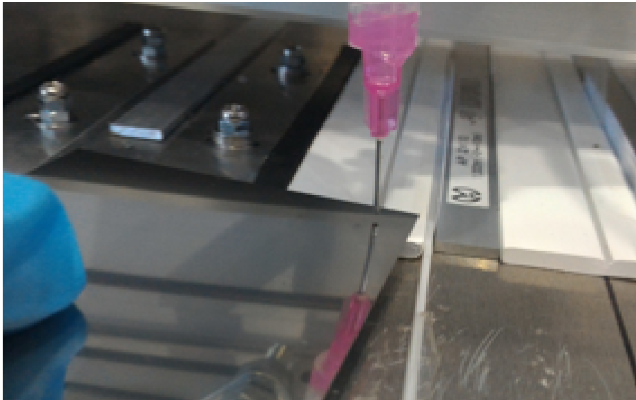
Figure 8.3.4: Aluminum board for adjusting the gap between the nozzle and the fiber
