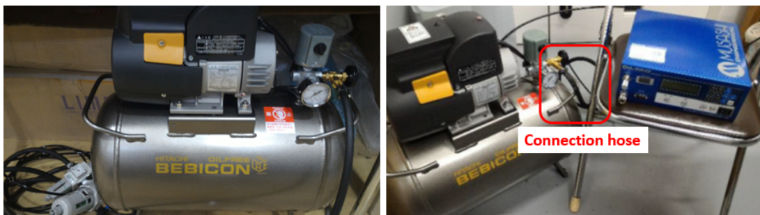
Figure 8.2.14: Air compressor : The right figure shows the connection with the dispenser.
