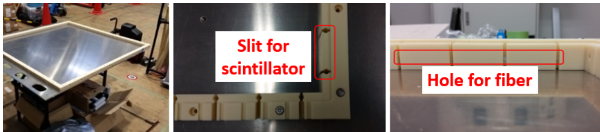
Figure 7.2.5: Set frames : Materials are made by ABS resin
