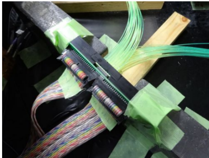
Figure B.2.13: Connection of the fiber bundle and MPPC
