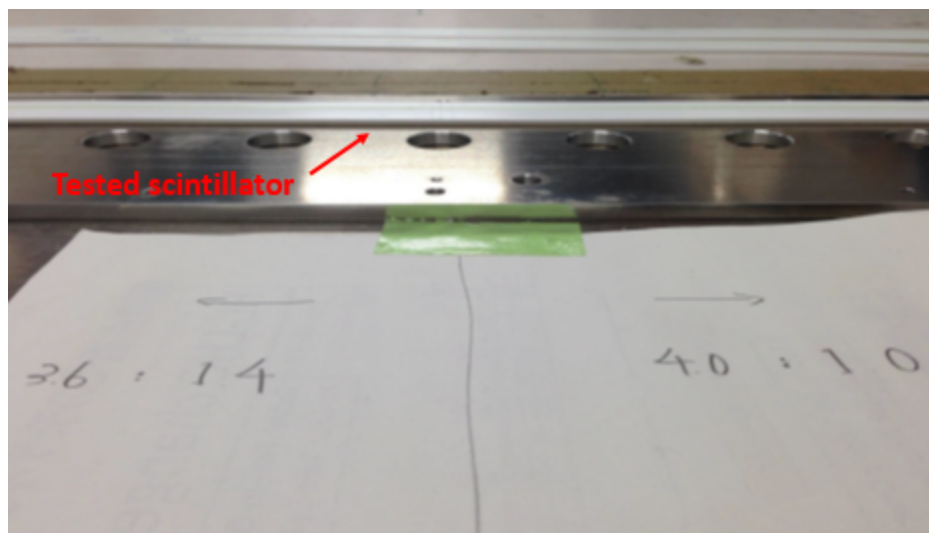
Figure 8.2.2: Setup for the cement test : On a scintillator, the half of it was glued with the fiber in the mass ratio of 3.6 per 1.4, and the other side in the original mass ratio.
