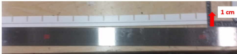
Figure 8.3.2: WAGASCI scintillator : It is a slightly distorted.
