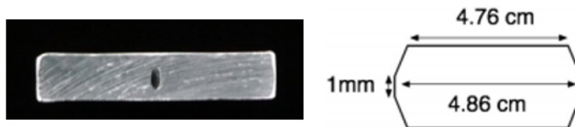
Figure 4.1.3: Sectioned picture and illustration of scintillator
