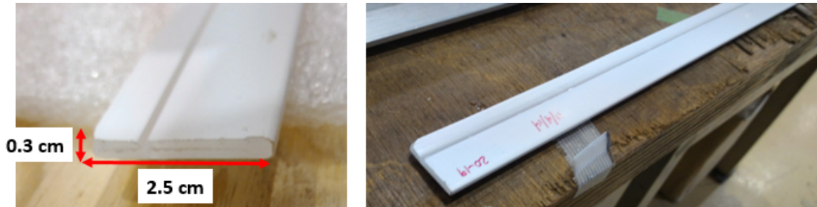
Figure 6.3.5: WAGASCI scintillator : There is a groove on the scintillator.
