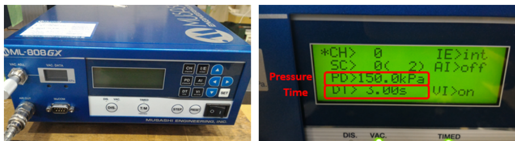
Figure 8.2.9: Dispenser : The right figure shows the control panel.
