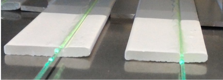
Figure 9.1.4: Cross sectional view of the scintillator : It is not a flat shape.
