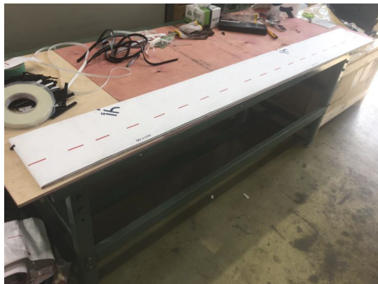
Fig. 5.4: A scintillator covered with Tyvek sheet.
