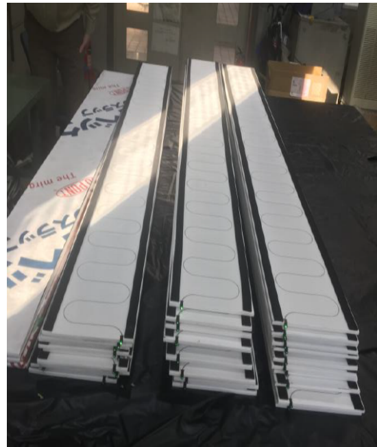
Fig. 5.3: A view of sponge rubber (left) and scintillators attached with the rubbers (right).
