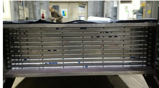
Fig. 5.5: Top view of SideMRD after installation of 80 scintillators.
